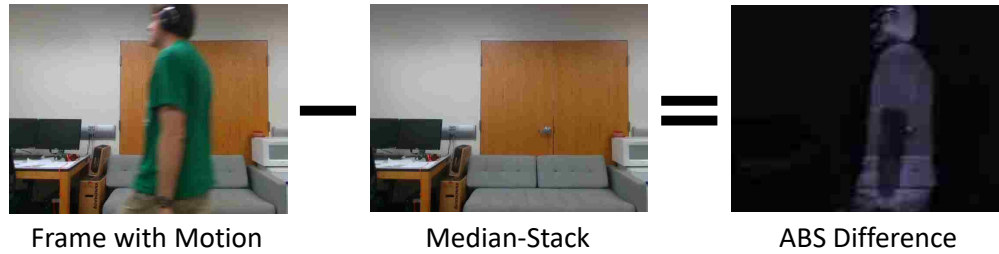
Figure 4.3: Motion removal. We remove frames with motion by taking the absolute difference of each frame with the median-stack image, and removing any frames that violate a threshold. ABS Difference colored here for clarity.
