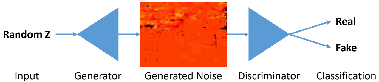
Figure 3.1: GAN diagram. The generator converts random noise into realistic-looking data, while the discriminator classifies that data as real or fake. In our case, the generator learns to produce realistic depth noise, while the discriminator determines if that noise looks real or not.
